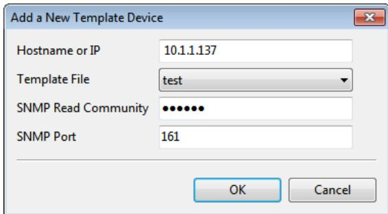
Specify the network device's IP or hostname, and select the “**test**” Template File from the drop-down list. Specify the SNMP read community and port, if they are different from the default values. The virtual sensors will be automatically added to the Template Device.
