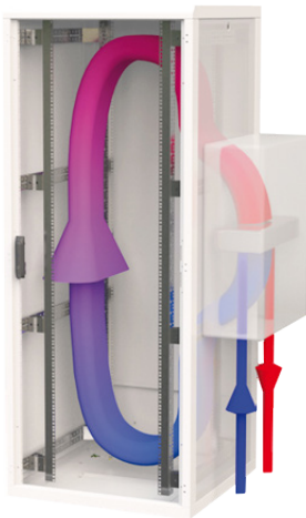
Air flow through the rack— CoolSpot CW WW version
