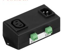
The PowerBox is designed to detect and control 110/230VAC voltage by turning on or off. The PowerBox can be controlled both voltage and voltage free. Suitable for remote server restart, controlling additional cooling or fan and many other functions.
