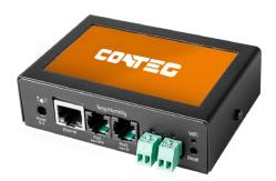
RAMOS Micro is a simple small solution for monitoring the environment of IT racks. With two new universal ports it can monitor up to 5 sensors (temperature, humidity, flood, pressure, CO2, etc.) and with 2 binary inputs it can detect other possible parameters such as door contacts, smoke, motion, flood detectors, etc. It supports PoE power supply and WiFi communication.
