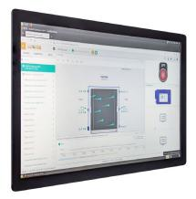
21,5" touch monitor with built-in computer (Linux OS). It can be used for remote access to CONTEG Pro Server (CPS) and other applications, or as a web kiosk. The monitor can be used to monitor current information in the data hall, e.g. for individual aisles or the entire data center.
